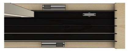
The inline return pulley is used when there is a minimum of 11/16" between the top of the panel and the head track. The lead panel will travel under the return pulley to the closed position. The inline pulley excepts only 3/8" belt and is typically used for systems under 20'.
