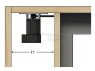
The motor is installed on either side of the stacking bi-part unit in the next available stud bay.
