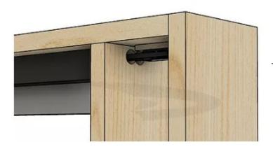
Two 1-1/8 holes will be drilled through the stud wall and the jamb to allow the belt to travel from the stud bay into the door unit.
