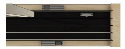
The inline return pulley is used when there is a minimum of 11/16" between the top of the panel and the head track. The lead panel will travel under the return pulley to the closed position.
