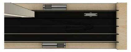
The inline return pulley is used when there is a minimum of 11/16" between the top of the panel and the head track. The lead panel will travel under the return pulley to the closed position. The inline pulley excepts only 3/8" belt and is typically used for systems under 20'.
