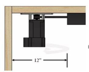
The motor can be installed on either side of the pocketing bi-part unit.
