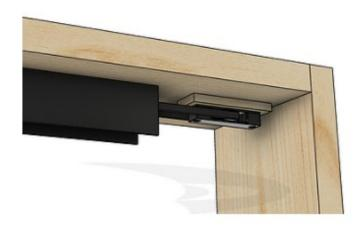
Like the motor, the return pulley will be installed in the center of the lead panel track, so we can attach the belt to both lead panels of the door unit.
