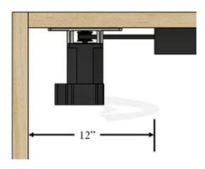
The motor will be installed on the pocket side of the one-way unit.
