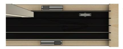
The inline return pulley is used when there is a minimum of 11/16" between the top of the panel and the head track. The lead panel will travel under the return pulley to the closed position.
